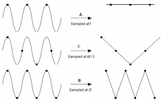
Only Case B (sampling twice over each cycle) correctly measures the signal.
