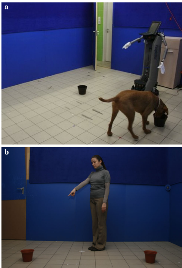
Fig. 1 a The customized PeopleBot mobile platform, which was equipped with a 5 degree of freedom robotic arm endowed with a four-fingered hand. b The human experimenter adjusted her movements to the physical abilities and constraints of the robot. The robot had only one moveable pointing arm, and thus, the human experimenter always used the same arm for pointing
