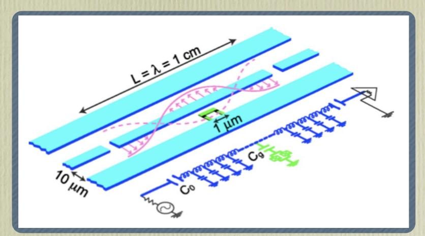
Cavity: Transmission line resonator (TLR)
