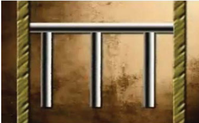
Section Diagram of Building Showing Wooden Interior Floor Supports and Exterior Brick Walls, CCTV video.
