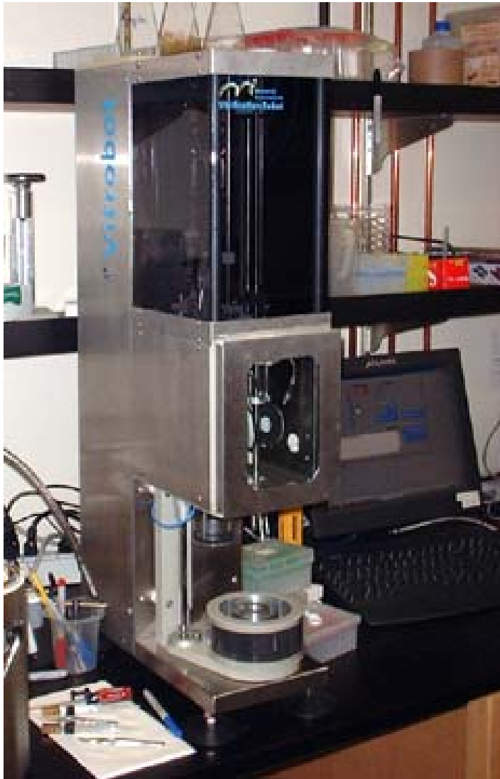
The Vitrobot™, produced by Maastricht Instruments, is computer controlled to simplify and automate the vitrification of liquid samples.
