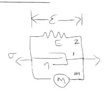
a) (15 points) Build a mathematical model from this diagram, to derive an equation for the strain of the fiber,  $\epsilon$ , vs the external stress applied to the fiber,  $\sigma$ .
