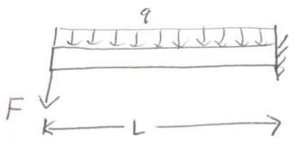
2. (30 points) A beam has length L, Young's modulus E, and a circular cross-section with radius r. What is the maximum deflection, v, of the beam in the situation below, and at what position x does this deflection occur? (you can assume small deflections)
