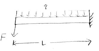
Need to find M(x) and V(x) to find ox & t, then Don't need to solve for support rxn if cut: M(x) + 9x = +x = 0; M(x) = - Fx - 2x2 = FFx - Fx -V(x)-9x-F=0, V(x)=-F-9x=-F-=x Allterms vogative, so extreme value at largest x:L M(L) = - FL - E= - FL - F/2 - - 3 FL Feils when 2 FL = N; or 9 FL = 2U or 3U F=2UH2W from shear or compression.
