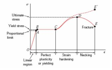
Finally, all materials fail above critical values. Different materials fail in different ways. **Brittle** materials are stiff and remain linear until they fail by sudden fracture, while ductile materials undergo an irreversible plastic deformation
