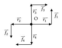
This requires that these two forces also have magnitude  $f = |a^2 \tau_{xy}|$ , so  $\tau_{xy}$  and  $\tau_{yx}$  are equal in magnitude. They must point in the direction shown above in order to be negative in sign. Finally, we note that this is applying a positive force to a positive face (+/+) for one and (-/-) for the other, so the sign must be positive. Thus,  $\tau_{yx} = \tau_{xy}$ .
