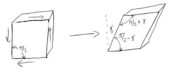
We define **shear strain** =  $\gamma$  to be the decrease in the angle between two positive faces. Note that when  $\tau > 0$ , this means  $\gamma > 0$ .
