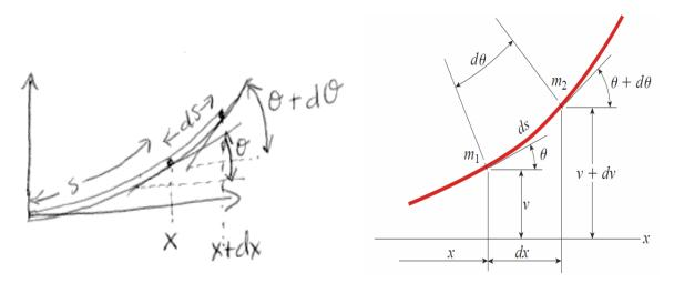
As in the diagram above, we consider a beam with tangent angle  $\theta$  at length s along the beam, with the neutral plane at position (x, v). At length s + ds along the curve, the neutral axis lies at position (x + dx, v + dv), and the tangent angle is  $\theta + d\theta$ .
