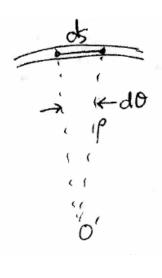
Next we consider the longitudinal strains from this bending. If the beam bends upward (M>0), then the upper region is under compression and the lower region under tension. We define the neutral plane as the surface within the beam that is not under compression or tension. We will learn later how to find this place, but for now, we will call the neutral plane y = 0.
