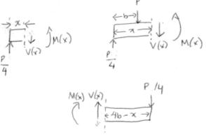
• To find the min and max of M(x), it is useful to draw the bending moment diagram. Each segment is linear in x, so we can just calculate M(0), M(b), M(2b), M(4b), which are the points between segments. For the internal points, we have two ways to calculate M(x). Since there is no couple , the two values should be the same. (If there were a couple, the two values should differ by  $M_0$ , the moment applied by the couple.) Thus,
