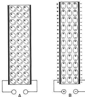
An electric field realigns the dipoles in a piezoelectric crystal
