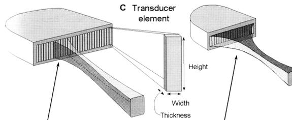
A subset of transducer elements activated
