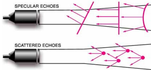
**Specular** - echoes originating from relatively large, regularly shaped objects with smooth surfaces. These echoes are relatively intense and angle dependent. (i.e. valves) - **Reflection from large surfaces**
