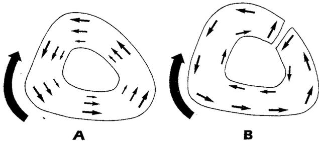
FIG. 1-43 Stress pattern in an open and closed section under torsional loading. **A.** In the closed section, all the shear stress resists the applied torque. **B.** In the open section, only the shear stress at the periphery of the bone resists the applied torque. (Adapted from Frankel and Burstein, 1970.)
