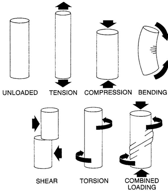
FIG. 1-10 Schematic representation of various loading modes.
