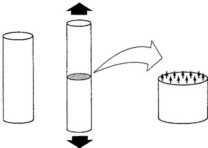
FIG. 1-11 Tensile loading.
