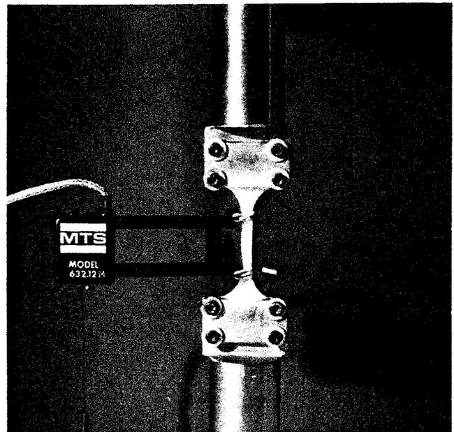
FIG. 1-5 Standardized bone specimen in a testing machine. The strain in the segment of bone between the two gauge arms is measured with a strain gauge. The stress is calculated from the total load measured. (Courtesy of Dennis R. Carter, Ph.D.)
