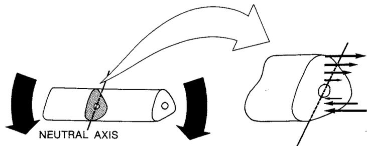
stresses and strains act on one side of the neutral axis, and compressive stresses and strains act on the other side (Fig. 1-23); there are no stresses and strains along the neutral axis. The magnitude of the stresses is proportional to their distance from the neutral axis of the bone. The farther the stresses are from the neutral axis, the higher their magnitude. Because bone is asymmetrical, the tensile and compressive stresses may not be equal.
