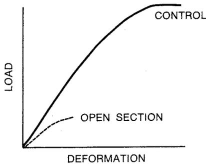
FIG. 1-44 Load-deformation curves for human adult tibiae tested *in vitro* under torsional loading. The control curve represents a tibia with no defect; the open section curve represents a tibia with an open section defect. (Adapted from Frankel and Burstein, 1970.)
