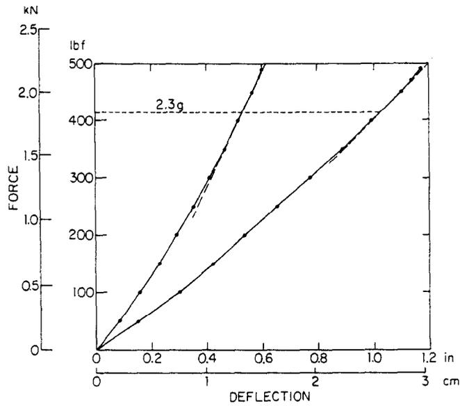
Fig. 2. (b) Force-deflection curves for two configurations of the experimental wooden track. Tangents fit to the 2.3g level give  $k_t = 13,333 \text{ lbf/ft}$  (195 kN/m) and  $6857 \text{ lbf/ft}$  (100 kN/m).
