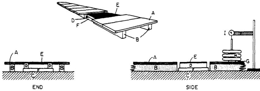
Fig. 2. (a) Three views of the experimental wooden track. A—plywood running surface, B, D—spruce supporting rails, C—concrete floor, E—phenolic resin board, F—force platform, G—aluminum plate representing the foot, H—weights, I—displacement gauge.
