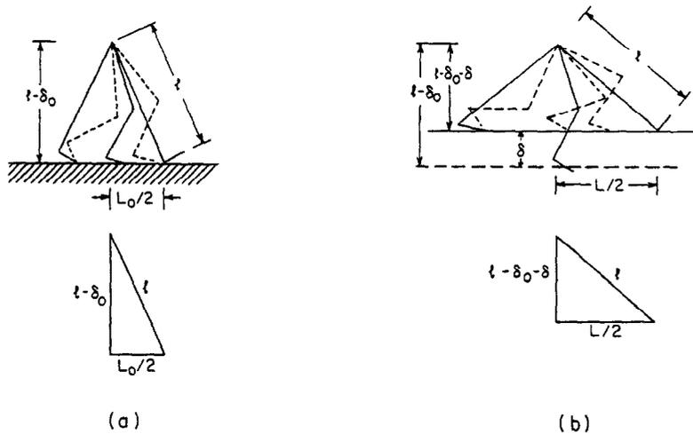
Fig. 5. Schematic of a step on (a) hard surface and (b) pillow track. Solid line shows the stance leg, broken line shows the swing leg moving forward. Because the foot descends a distance  $\delta$  into the pillows, the step length on the pillow track is necessarily greater.
