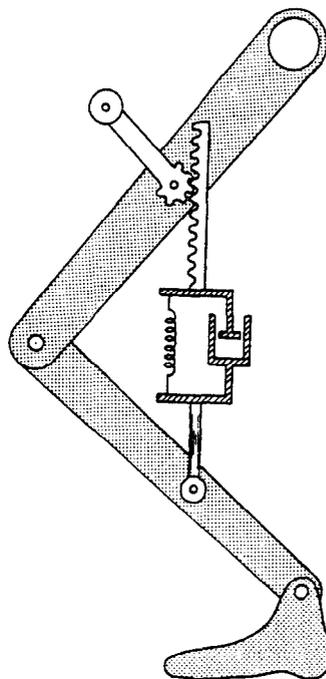
Fig. 1. Schematic representing the separate role of descending commands (rack-and-pinion) and muscle properties plus local reflexes (damped spring). The motion of the rack and pinion element determines the influence of track stiffness on step length. The runner's mass and the damped spring determine the influence of track stiffness on ground contact time.
