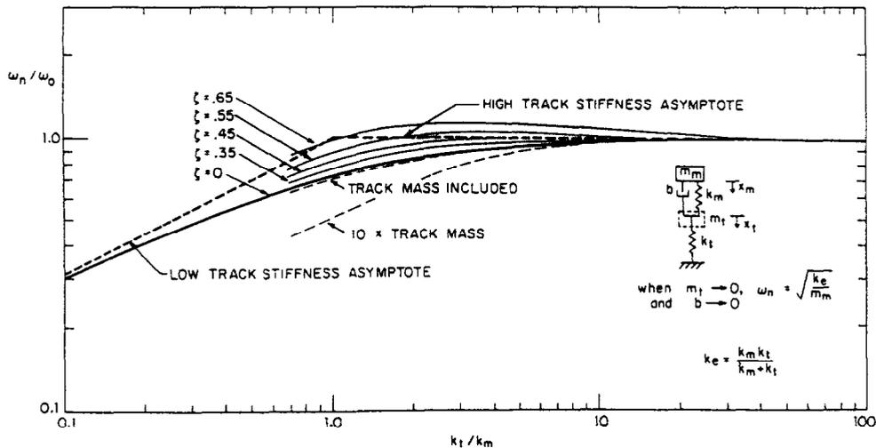
Fig. 3. Normalized natural frequency vs normalized track stiffness. The inset shows the damped two-mass, two-spring system. Heavy line shows zero damping, zero track mass.
