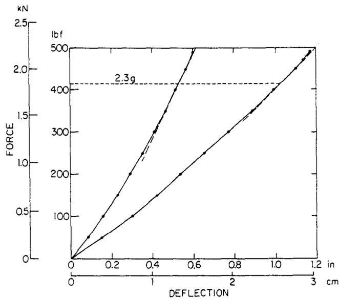
Fig. 2. (b) Force-deflection curves for two configurations of the experimental wooden track. Tangents fit to the 2.3g level give  $k_t = 13,333 \text{ lbf/ft}$  (195 kN/m) and  $6857 \text{ lbf/ft}$  (100 kN/m).
