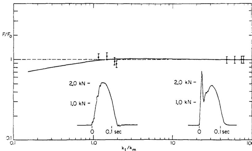
Fig. 9. Normalized average foot force vs normalized track stiffness. Solid line shows theory, solid points show average force platform results for each of four subjects. Insets show how the initial force transient experienced on hard surfaces is abolished on the experimental wooden track.
