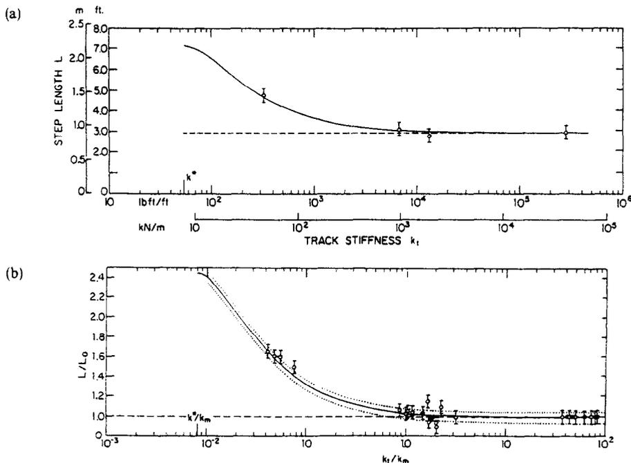
Fig. 7. Step length vs track stiffness. The solid line shows the theoretical prediction. (a) Subject M.F. alone. (b) Dimensionless plot showing all 8 subjects.
