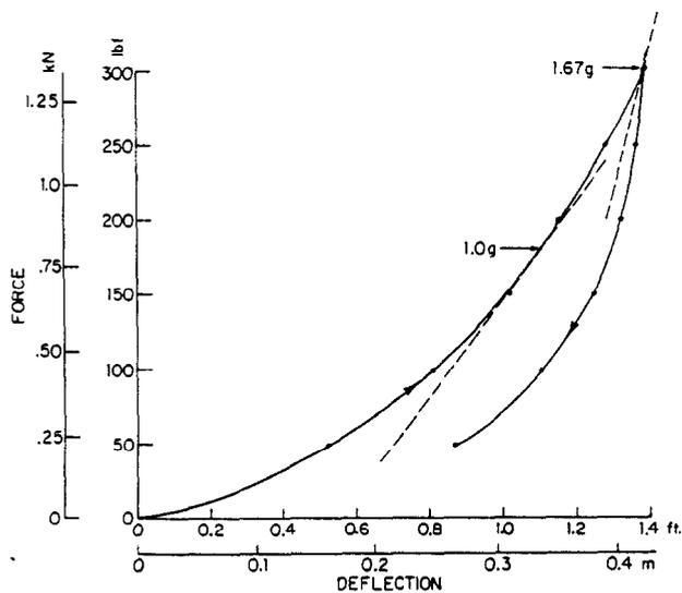
Fig. 2. (c) Force-deflection curves for the foam rubber pillow track, showing 1.0g and 1.67g tangents, which give  $k_t = 320 \text{ lbf/ft}$  (4.67 kN/m) and  $985 \text{ lbf/ft}$  (14.4 kN/m).
