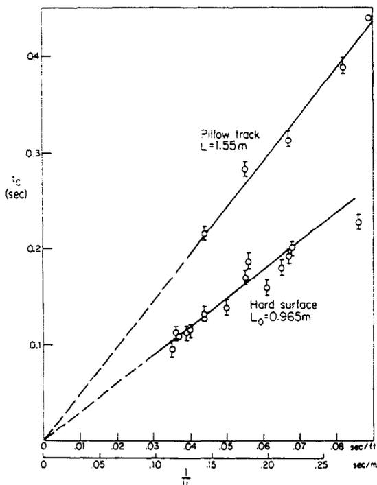
Fig. 6. Ground contact time  $t_c$  vs inverse running speed  $1/u$ , for runner M.F. The straight lines through the origin show that an individual's step length is constant, independent of the running speed, on a particular surface. Step length is greater on the pillow track than on the hard surface. Error bars show maximum uncertainty due to film reading.
