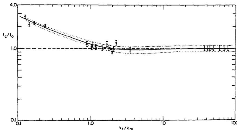
Fig. 8. Normalized foot contact time  $t_c/t_o$  vs normalized track stiffness, assuming damping ratio  $\zeta = 0.55$ . Open circles show data produced by film analysis; closed circles show force platform data. Error bars show limits of uncertainty due to film and oscilloscope reading; dotted lines are one standard deviation above and below the theoretical line.
