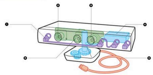
Microphone array Four mics pinpoint where voices or sounds are coming from while filtering out background noise.
