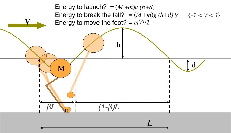
Goal: compute the power (rate of energy expenditure) as a function of size (M,m) and gait (jumpiness)  $j = (1-\beta)/\beta$ Total Energy  $= (1+\gamma)(M+m)\frac{g^2 L^2(1-\beta)}{8V^2} + mV^2/2$
