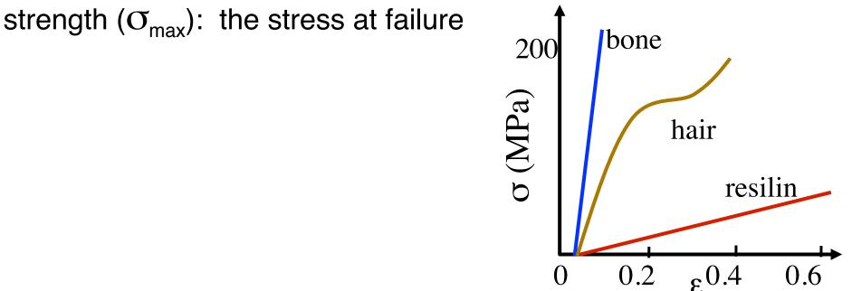
stress ( $\sigma$ ) : the distribution of force over an area strain ( $\epsilon$ ): a dimensionless measure of length change stiffness (*E*): the change in stress required for a change in strain (the slope of a stress-strain curve) a material property
