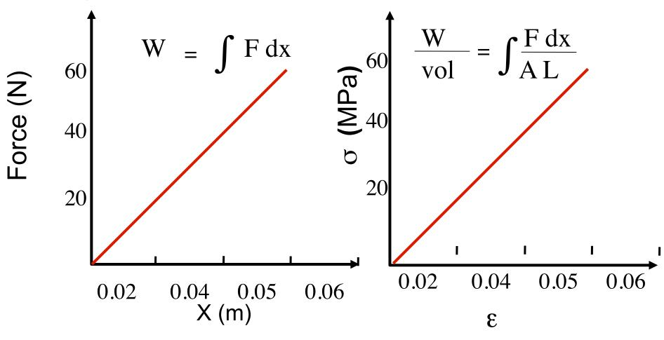
The energy imparted is the mechanical strain energy
