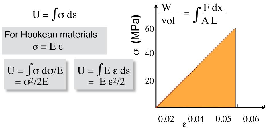
The energy imparted is the mechanical strain energy that can be returned or be so great as to break the material
