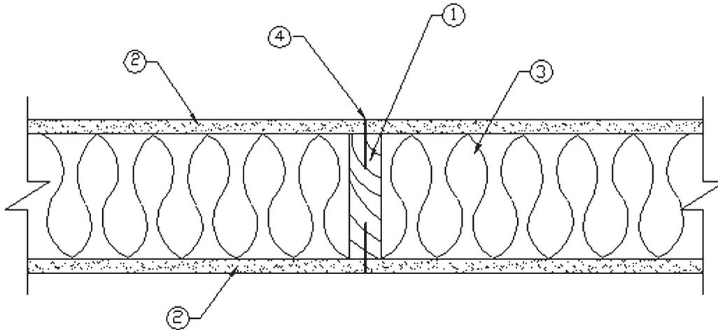
1. **Framing:** Nominal 2x6 wood studs, spaced 16 in. o.c., double top plates, single bottom plate.
