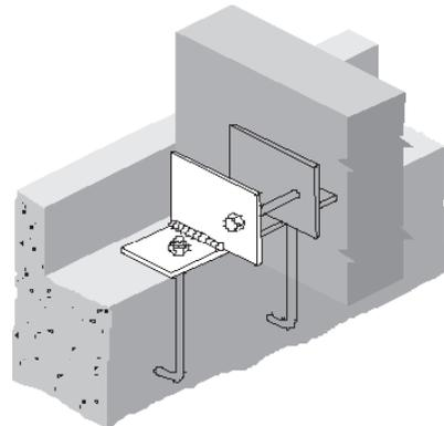
34A. This sloped bearing with a beam that is not fully supported may also split under load. **THIS DETAIL IS NOT RECOMMENDED!**
