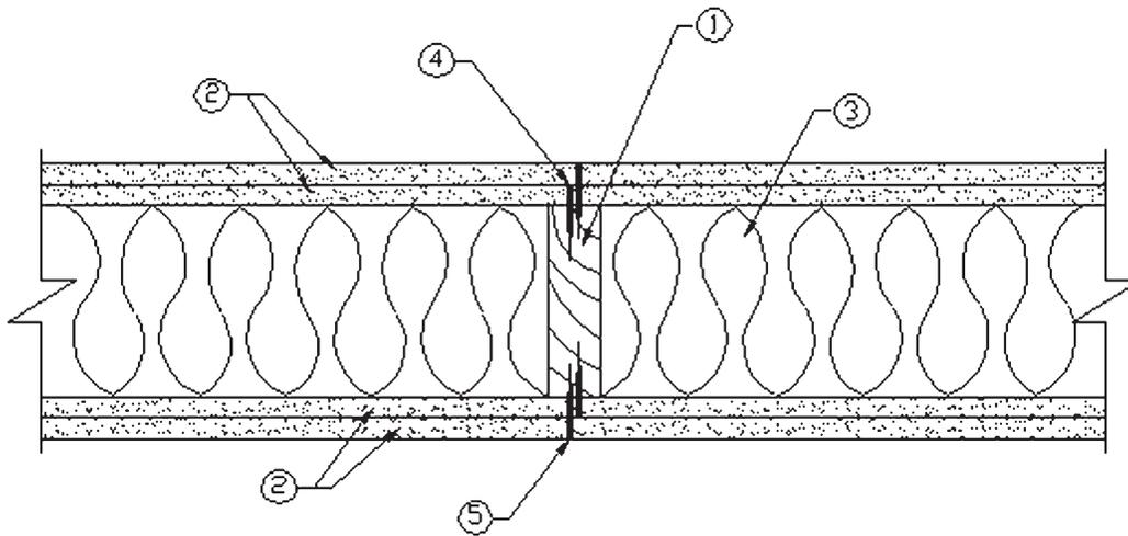
1. **Framing:** Nominal 2x6 wood studs, spaced 24 in. o.c., double top plates, single bottom plate.
