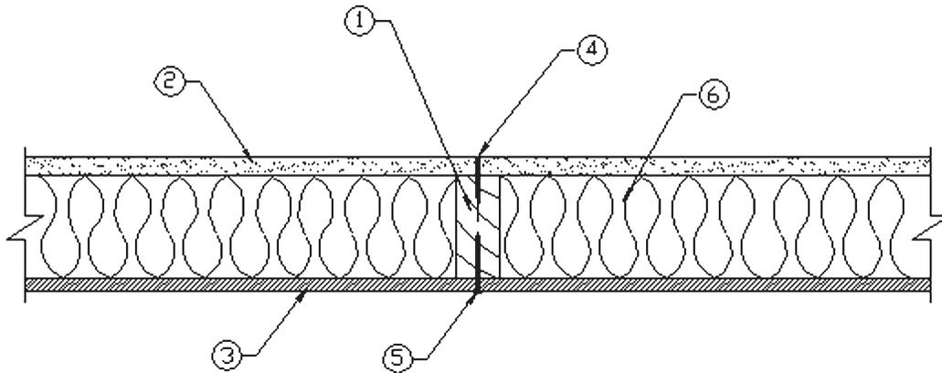
1. **Framing:** Nominal 2x4 wood studs, spaced 16 in. o.c., double top plates, single bottom plate.
