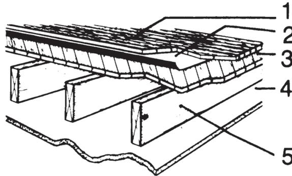
1. Nominal 1 in. wood flooring or 19/32 in. T&G plywood underlayment (single floor). Oriented strand board (OSB) panels are permitted for certain designs.
