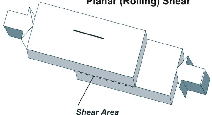
**Table M9.2-3 Wood Structural Panel Planar (Rolling) Shear Capacities**
