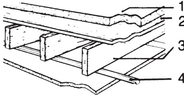
1. 1-1/2 in. lightweight concrete or minimum 3/4 in. proprietary gypsum concrete floor topping. Building paper may be optional and is not shown.
