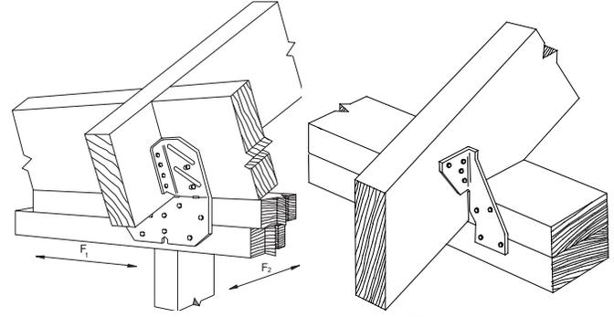
Seismic and Hurricane Ties
