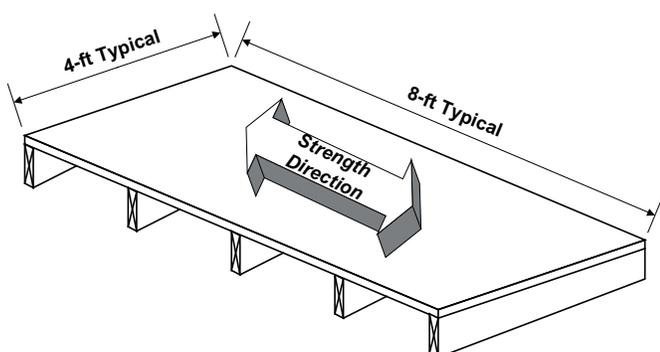
Designers must specify wood structural panels by the span ratings, nominal thicknesses, grades, and constructions associated with tabulated design recommendations. Exposure durability classification must also be identified.
