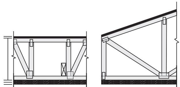
**Two-Hour Fire Resistive Truss Designs:**
