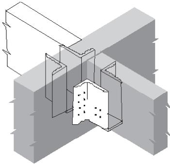
15. Deep members may be supported by fairly shallow hangers – in this case, through-bolted with shear plates. Clip angles are used to prevent rotation of the top of the suspended beam. Note that the clip angles are not connected to the suspended beam – doing so would restrain a deep beam from its natural across-the-grain shrinking and swelling cycles and would lead to splits.
