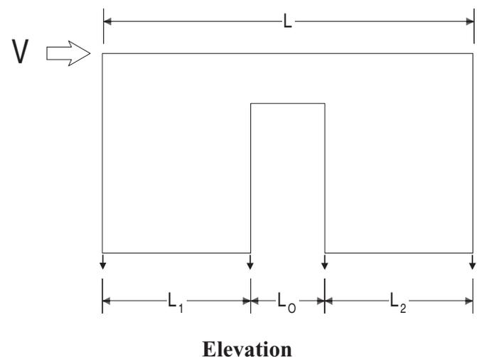
$$\text{Unit shear above opening} = \frac{V}{L} = v_a$$
