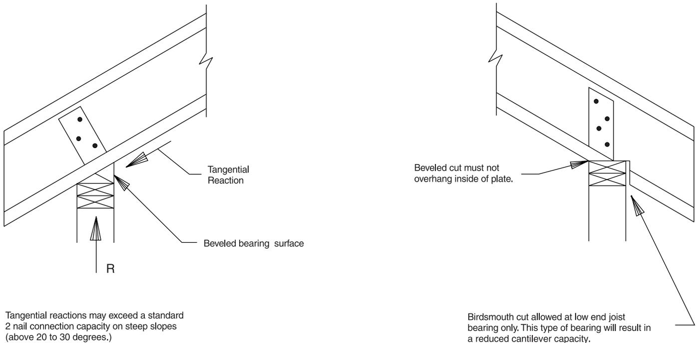
For the high end support, bottom flange bearing in a suitable connector or on a beveled plate is recommended. When slopes exceed 30°, straps or gussets may be needed to resist the tangential component of the reaction.
