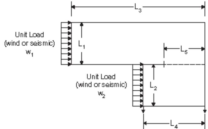
$$\text{Unit shear along } L_3 = \frac{W_1 L_1}{2L_3}$$
