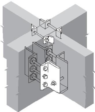
16. Concealed connections similar to detail 5. The suspended beam may be dapped on the bottom for a flush connection. The pin may be slightly narrower than the
