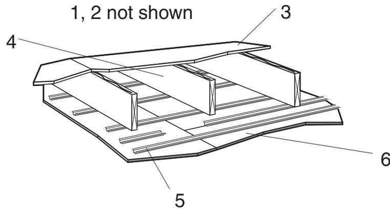
1. 1-1/2 in. lightweight concrete or minimum 3/4 in. proprietary gypsum concrete floor topping.
