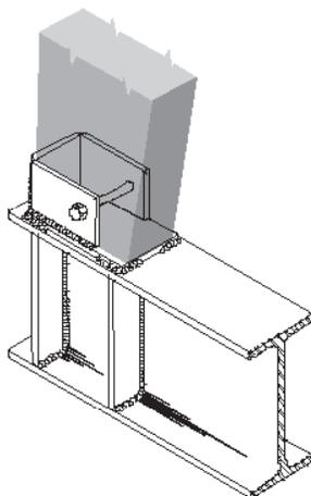
27. Similar to detail 25. This more rigid connection is suitable for spans where arch rotation at the base is small enough to not require the rotational movement permitted in detail 25. Note that, although the shoe is “boxed” a weep slot is provided at the inside face.
