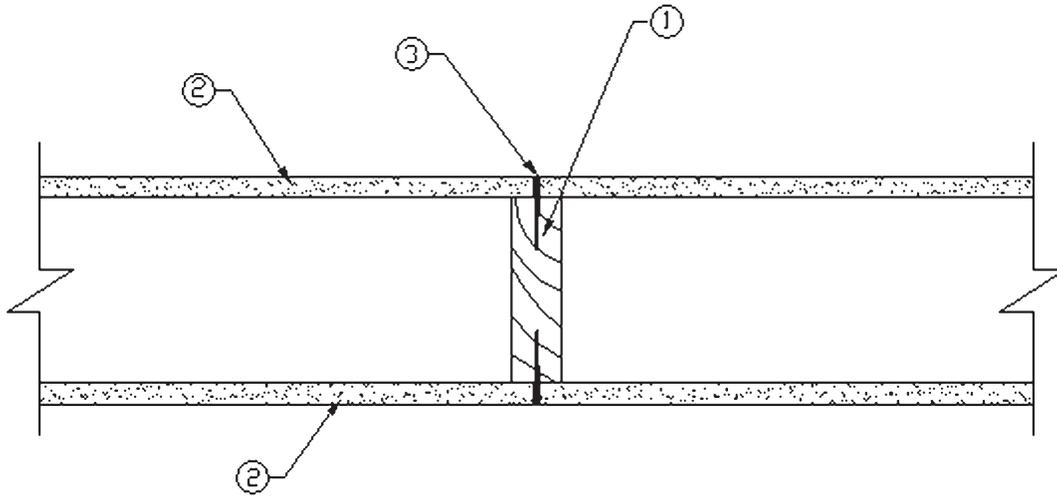
1. **Framing:** Nominal 2x6 wood studs, spaced 16 in. o.c., double top plates, single bottom plate.
