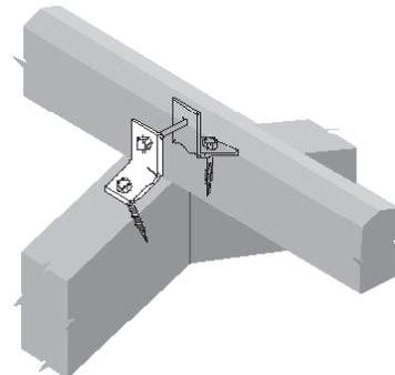
20A. Similar to detail 19, but with the segments of the ridge purlin set flush with the other framing.
