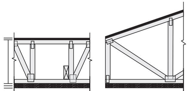
**90-Minute Fire Resistive Truss Designs:**
