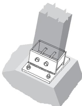
28. For very long spans or other cases where large rotations must be accommodated, a true hinge connection may be required.
