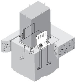
*Full-depth side plates.* It is sometimes easier to fabricate connections for deep beams from large steel plates rather than having to keep track of more pieces. Lack of attention to wood's dimensional changes as it "breathes" may lead to splits.
