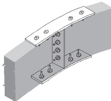
30. Similar to detail 29. Connectors on side faces may be easier to install, but forces are higher because moment arm between steel straps is less than in detail 29.
