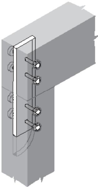
6. Custom welded column caps can be designed to transfer shear, uplift, and splice forces. Note design variations to provide sufficient bearing area for each of the beams and differing plate widths to accommodate differences between the column and the beam widths.
