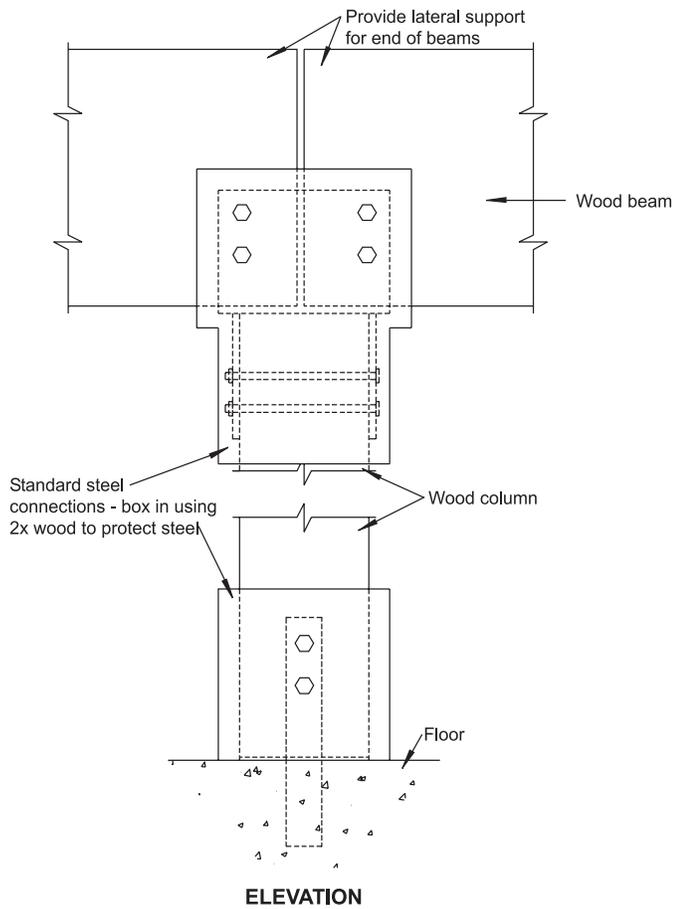
**Figure M16.3-6 Beam to Girder - Concealed Connection**
