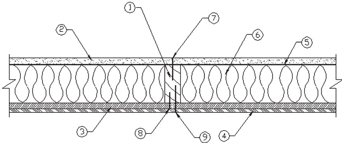
1. **Framing:** Nominal 2x4 wood studs, spaced 16 in. o.c., double top plates, single bottom plate.
