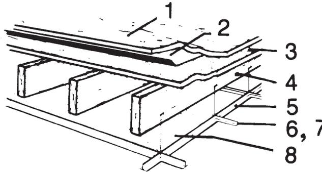
1. Nominal 19/32 in. T&G plywood underlayment (single floor). Oriented strand board (OSB) panels are permitted for certain designs.
