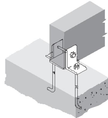
3. Similar to detail 1 with slotted holes to accommodate slight lateral movement of the beam under load. This detail is more commonly used when the beam is sloped, rather than flat.
