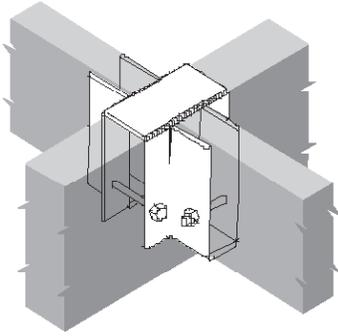
14. Face-mounted hangers are commonly used in beam to beam connections. In a “cross” junction special attention is required to fastener penetration length into the carrying beam (to avoid interference from other side).
