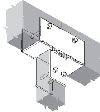
7. Combinations of steel angles and straps, bolted and screwed, to transfer forces.
