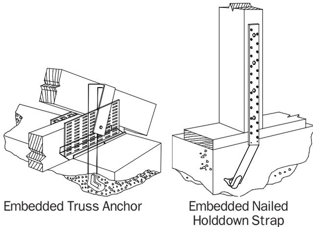
Embedded Truss Anchor
