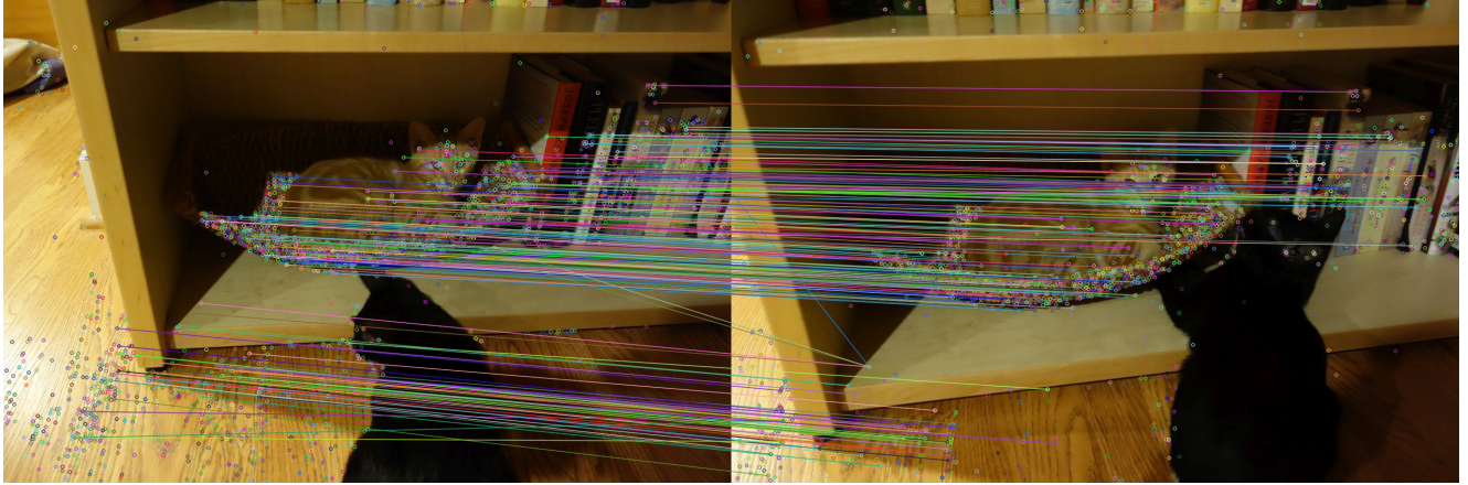
Figure 1. Example of SIFT keypoint matching on images of furry creatures. The top 200 matches are displayed. With SIFT matching six incorrect matches are found.
