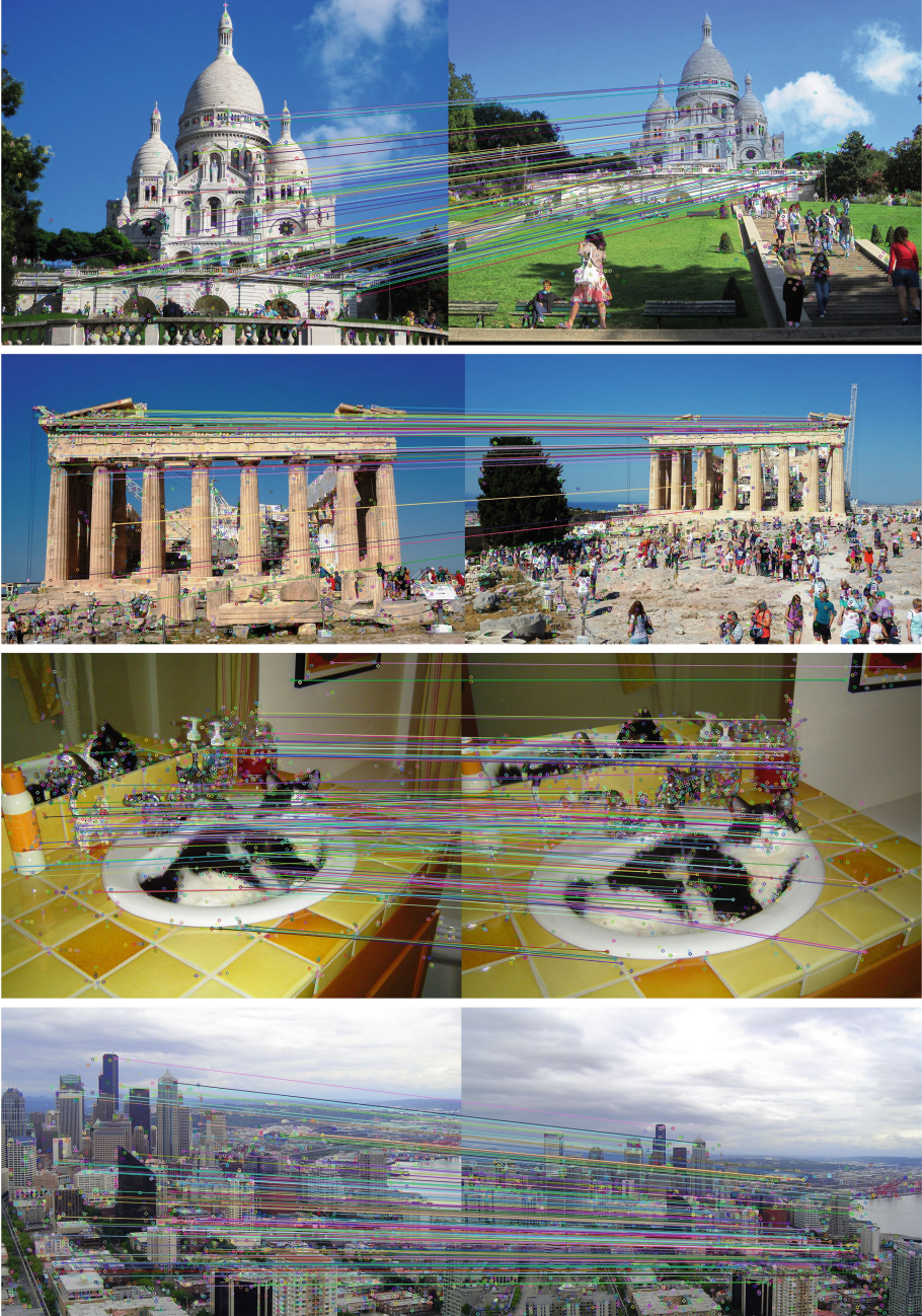
Fig. 2. Matching examples. The top matches detected using CNN3+HoNC+SIFT on four example pairs. The top pair shows the 100 best matches. The other pairs show the 200 best matches.
