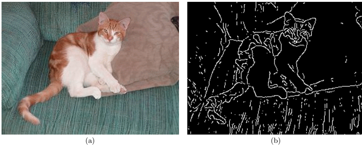
Figure 4: Edge detection is performed with linear filtering, followed by thresholding, and non-maxima suppression. (a) Input image. (b) Output image.
