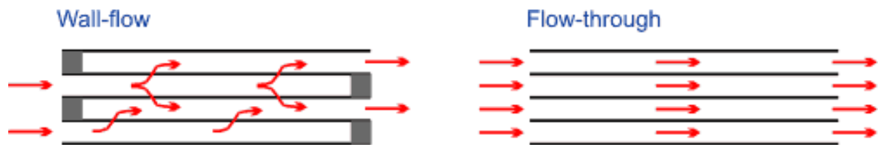
Figure 2. Wall-Flow and Flow-Through Substrates: Flow Pattern
