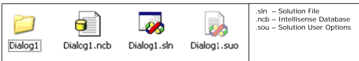
Figure 4. Files created inside the Dialog1 solution folder when the Create directory for Solution checkbox is selected.
