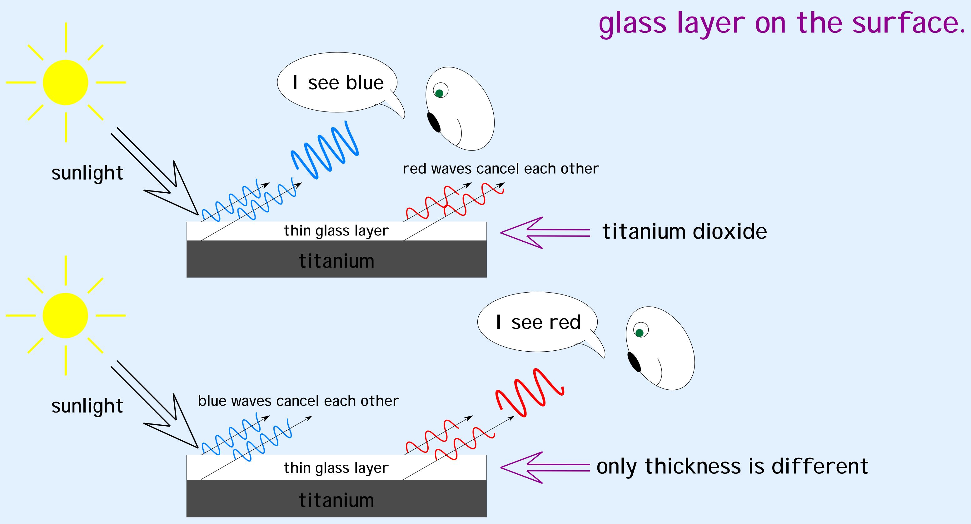
We'll create the thin glass layer using electrochemistry to oxidize titanium (Ti) into titanium dioxide (TiO<sub>2</sub>)
