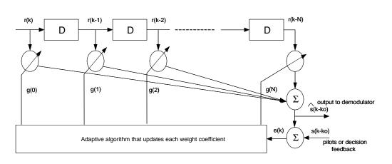
An adaptive channel equalizer has the following structure.
