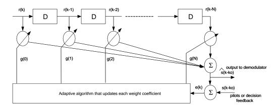
In most cases, a training sequence (or pilot sequence) is inserted periodically during data transmission. This particular set of symols  $\{s_k\}$  are therefore known to the receiver and thus can be used to train the equalizer (i.e., update its cofficients).
