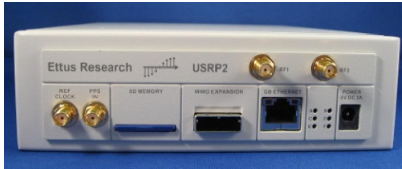
Figure 2: Front panel of a Universal Software Radio Peripheral, Version 2 (USRP2) SDR platform.
