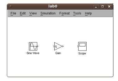
Figure 7: Gathering all the necessary blocks for the model.
