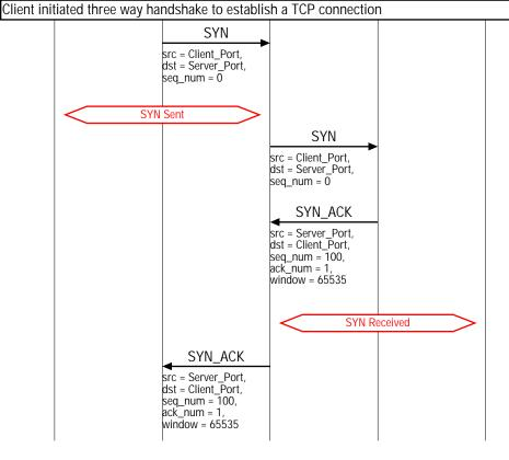
Server sets the SYN and the ACK bits in the TCP header. Server sends its initial sequence number as 100. Server also sets its window to 65535 bytes. i.e. Server has buffer space for 65535 bytes of data. Also note that the ack sequence numer is set to 1. This signifies that the server expects a next byte sequence number of 1
