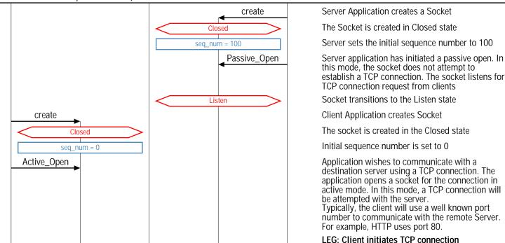
Client sets the SYN bit in the TCP header to request a TCP connection. The sequence number field is set to 0. Since the SYN bit is set, this sequence number is used as the initial sequence
