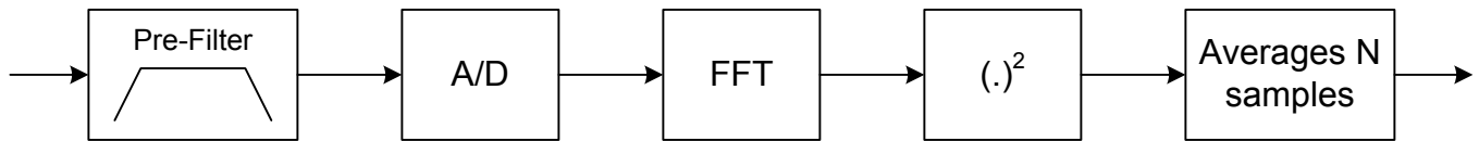
Figure 7: Schematic of an energy detector implementation employing pre-filtering and a square-law device.
