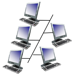
shared wire (e.g., cabled Ethernet)
