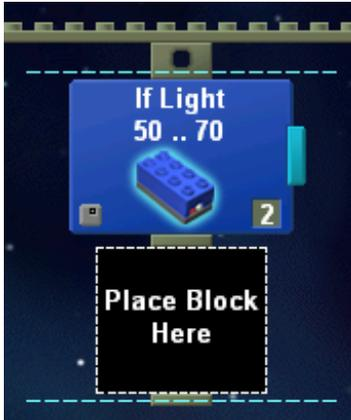
Use the view button on your RCX to determine the light intensity in the location your robot will be running. Use these values to set the range for dark and bright. This process is called calibration and you should do it often since light conditions change all the time.
