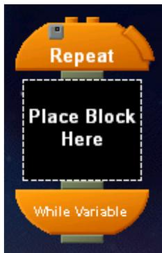
Execute a series of commands as long the variable counter is within a certain range. Once the counter exceeds the predefined value, the program exits the loop. Again, you can instead use a light or touch sensor here.
