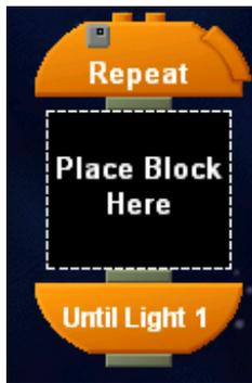
Execute a series of commands as long the light sensor reading is outside a certain range. Once the light enters the predefined range, the program exits the loop. This is just an example of a repeat command. You can use a touch sensor or a variable counter as well here.
