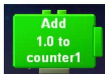
These commands can be used to keep track of the number of times certain events occur (for example how many times the touch sensor is pressed or the robot has turned). At the beginning of the program, the counter is always 0. To use, simply place the "Add to Counter" button on top of the command(s) you want to count. It is a good idea to reset the counter when you are done using it (so if later in the program, the robot needs to count something else, it will start from 0).
