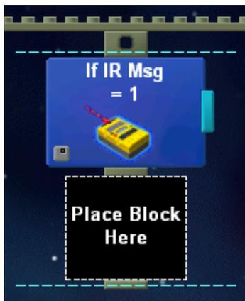
This command allows you to program your robot to do certain commands when it receives an infrared signal.
