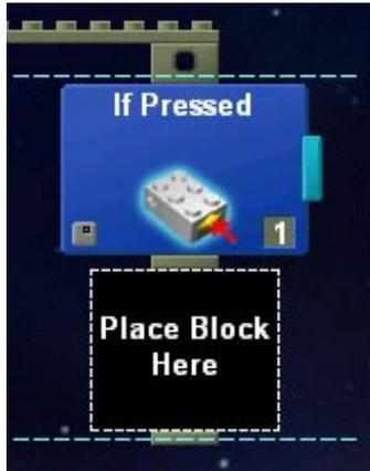
Select the port (1-3) that the touch sensor is attached. Usually it is easiest in a complicated program to only write code for the "Press" condition.
