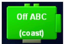
Turns the motors off. Note that there is a difference between the coast and break option. Braking means that in addition to stopping the motor, brakes are applied to prevent the robot from moving. Coasting stops the motor but allows the robot to still move until it stops by itself or runs into something.
