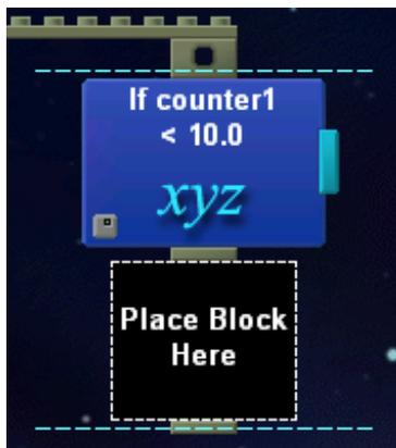
The counter can be used to program the robot to do certain tasks after or before a specific set of events occurs. For
