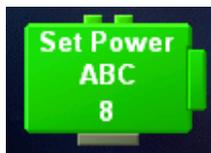
This is the first command that you should use in your program. This command sets the power level for the motors (1 is usually too low, 8 is the maximum). Remember that the battery power affects the speed of the motors (i.e. 8 can be really slow if your batteries are weak).
