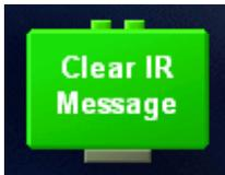
This command clears out any previously received message from another RCX. Note that you have to clear out the current message in order to be able to receive a new message. For example, in your wheelchair program, you have to stop after receiving signal "1" from the master controller. You should start moving again after receiving signal "2". So, in order to be able to receive message "2", you should clear message "1" first.
