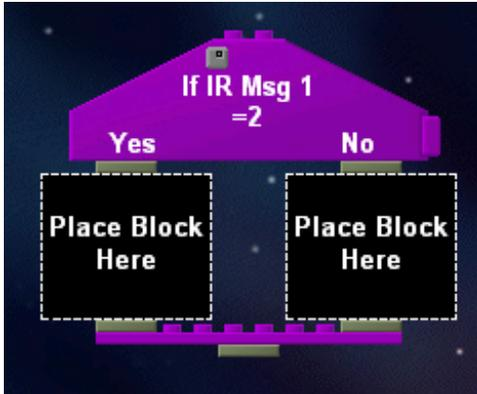
This is a conditional command. If the robot receives an IR message "2", the left set of commands are executed. If the robot receives an IR message of "1", the right set of commands are executed.
