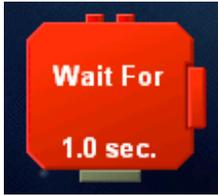
Does not mean stop! Instead causes the robot to wait a specific period of time before executing the next command.
