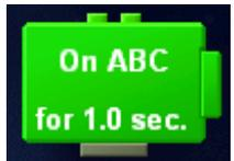
Allows the robot to move for a specific time period (in seconds).
