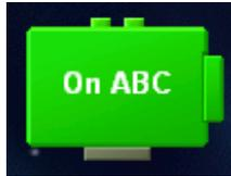
Turns motors (connected to ports A, B, or C) on (i.e. moves robot forward or backwards). The motors are on until you turn them off using the **Off** command below.
