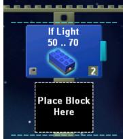
Use the view button on your RCX to determine the light intensity in the location your robot will be running. Use these values to set the range for dark and bright. This process is called calibration and you should do it often since light conditions change all the time.
