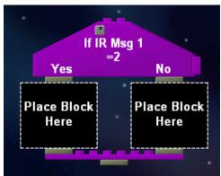
This is a conditional command. If the robot receives an IR message "2", the left set of commands are executed. If the robot receives an IR message of "1", the right set of commands are executed.
