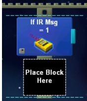
This command allows you to program your robot to do certain commands when it receives an infrared signal.
