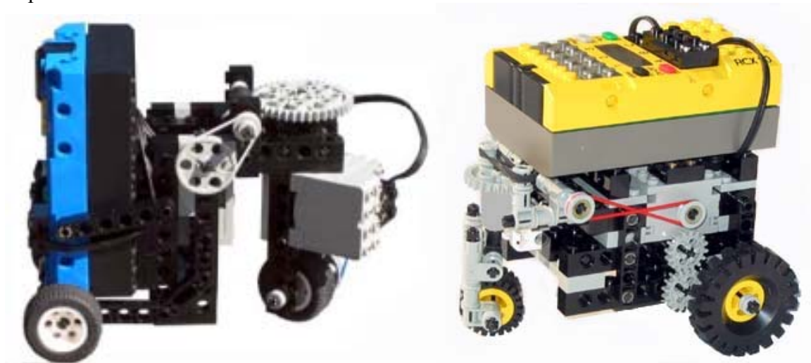
Figure 5-16. Tricycle Drive (Left) and Steering Drive (Right) Robots Look Similar
