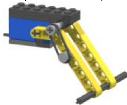
Figure 4-12. A Bumper that Uses the Rotation Sensor
