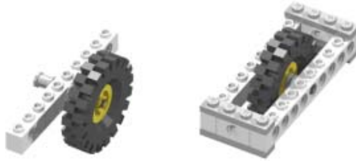
Figure 3-12. Cantilevered and Fully Supported Wheels
