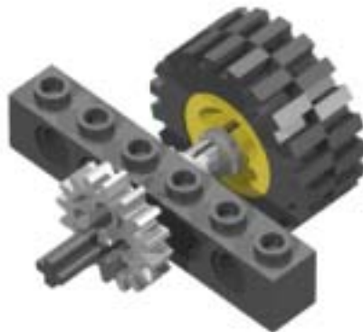
Figure 1-8. A Typical Driven Wheel Assembly
