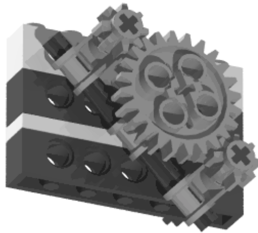
Figure 2-7. Circumventing Diagonal Gear Spacing Restrictions
