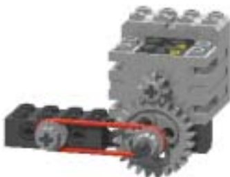
Figure 4-6. Using a Pulley to Increase Drag
