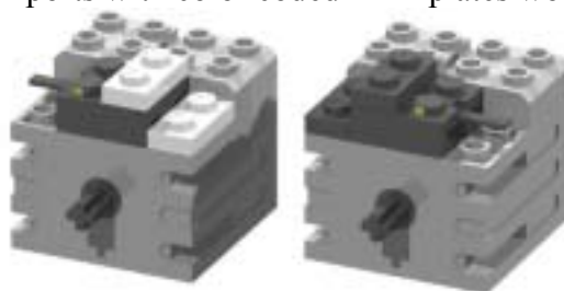
Figure 4-7. Using Color Coding to Document Proper Connector Orientation
