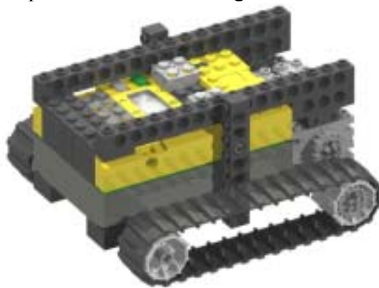
Figure 4-8. Strengthening Motor Mounts with Cross Bracing
