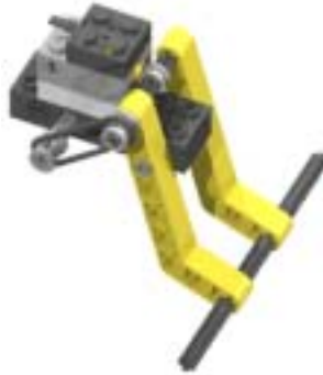
Figure 4-13. A Normally Closed Bumper Design
