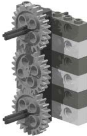
Figure 2-5. Circumventing Vertical Gear Spacing Restrictions
