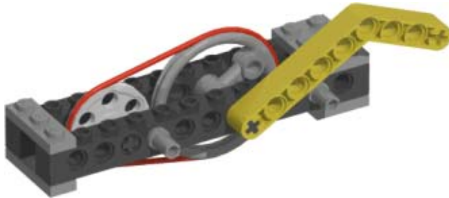
Figure 2-31. Using Pulleys to Limit Torque
