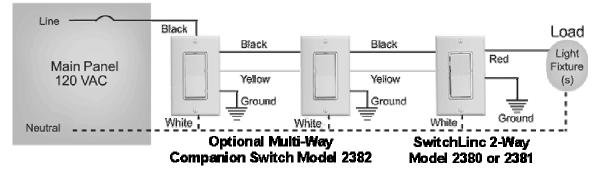
Using 2 SwitchLincs to Create a Virtual 3-Way Circuit
