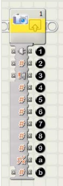
1. Port number to which NXTCam is supposed to be connected.
