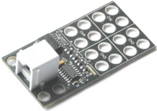
RXMux allows you to connect upto 4 RCX style sensors to NXT.
