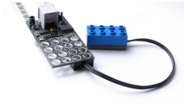
Picture above shows RCX Light sensor connected to RXMux.
