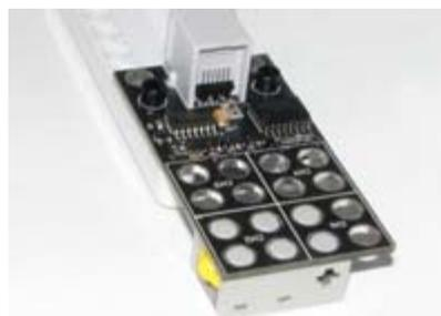
ensure to connect all four electric studs of Touch sensor to RXMux, as shown in adjacent picture.
