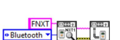
**Tip:** When you select a new VI such as **Create NXTObject** in this case and place it next to the relating VI icon, try to move it closer to the relating VI icon and you will find that LabVIEW will connect the corresponding ports for you.
