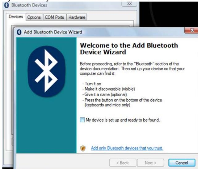
3. Press and hold **1** and **2** buttons of Wiimote at the same time for a while until you see the LEDs flash on and off. Check the **check box** of dialog and click **Next**.
