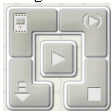
The controller has five buttons. The controller buttons work only if a NXT brick is connected by Bluetooth or a USB cable to a computer running the NXT environment.
