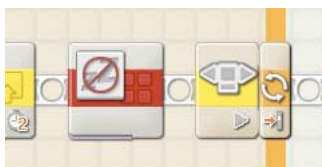
Fig 1-9: The Keep Alive block inside the main Loop, so it is executed each time through
