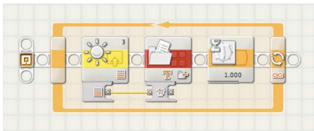
Fig 1-1: a minimal datalogging program. The Light Sensor block is configured to not generate light (uncheck the “Function” checkbox) and the File Access block is set to Write a number
