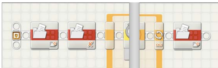
Fig 1-5: some File Access blocks, all with the “DLog” filename, to close, delete, and finally
