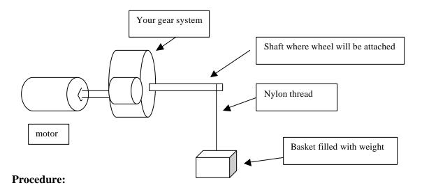
To measure the torque, attach a weight (measure the weight on a scale before begin the test) to the shaft where you will put the wheel using a nylon thread. Apply power to the motor (at maximum level), and the thread will begin to wind around the shaft. To find the maximum torque delivered by the system, you gradually increase the weight until the thread stop winding around the shaft.
