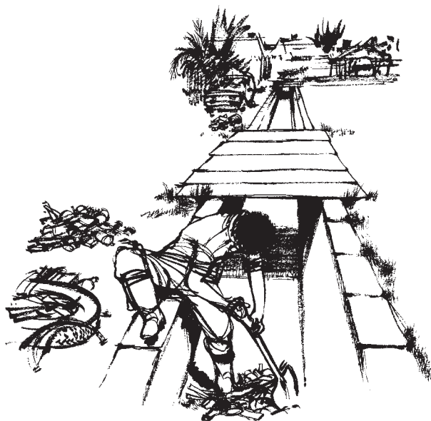
Fig. 1.128 Dirt, debris and other obstacles in drainage systems should be removed to allow the water to flow freely.
