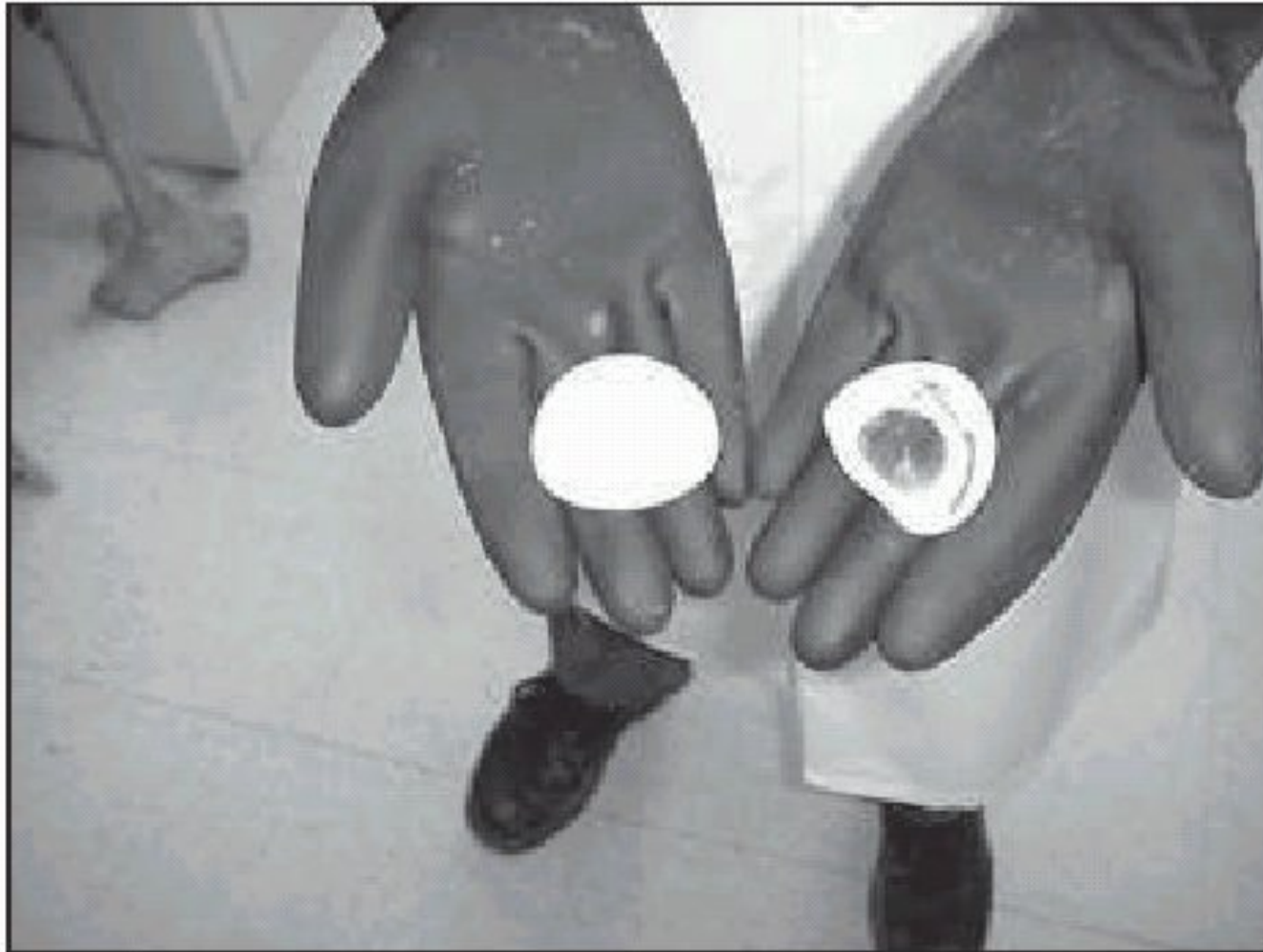
Figure 1. A polyvinyl chloride coated nylon before and after exposure to dimethylformamide. (Photo courtesy of Intertek Testing Services, Cortland, New York.)
