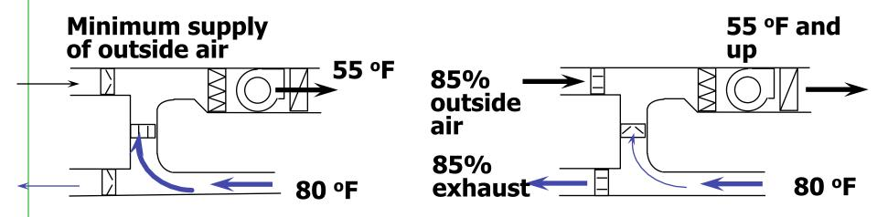
Normal Operation Outside air dampers are positioned to provide the minimum outside air
