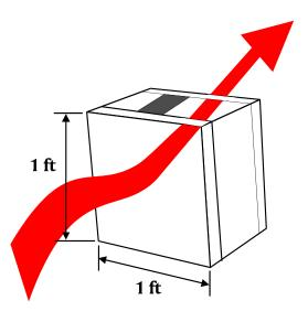
U-Value is the rate of heat flow in Btu/h through a one ft<sup>2</sup> area when one side is 1°F warmer
