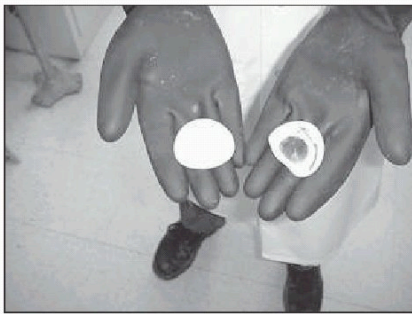
Figure 1. A polyvinyl chloride coated nylon before and after exposure to dimethylformamide. (Photo courtesy of Intertek Testing Services, Cortland, New York.)
