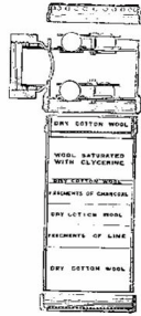
Figure 2.3 Tyndall and Shaw "smoke can" 5
