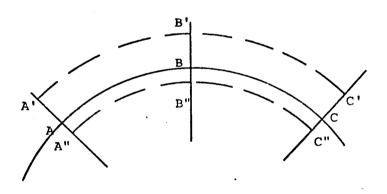
Using the distance W at each cross-section the designer should scale off W on the plan view. These are the points A', A", etc. Then the distances A'B', A"B", B'C', B"C" can be scaled off. These revised distances between the cross-section end areas are now used in the earthwork volume computation.
