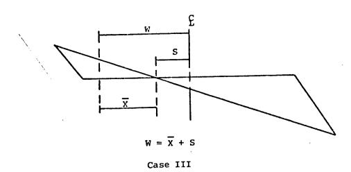
At each cross-section that lays on a horizontal curve the designer needs to determine the distance W for both the cut and fill sides:
