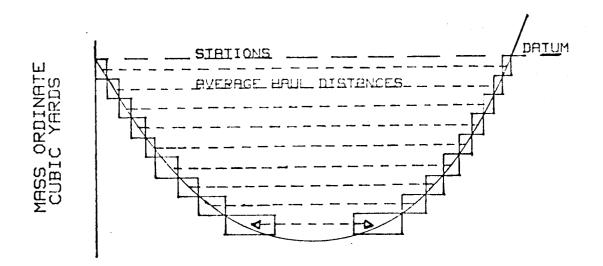
Alternate computational methods of determining the haul are available. However, they are tedious and are usually destined for computer solution.
