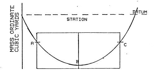
The vertical distance on the mass diagram between station A and station B is the yardage of  $\frac{2}{2}$  generated between the two stations.
