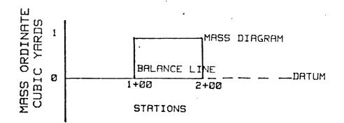
The simple analysis of this mass diagram shows that one cubic yard of excess excavation is generated at station 1+00 and is placed where there is a shortage of embankment at station 2+00. There is
