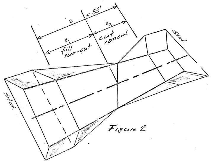
For lack of a better method, a simple pro-ration system is usually used. Refer to the sample EARTHWORK QUANTITY SHEET for the data in the following example.
