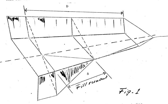
A similar distance can be figured for the cut-fill to through fill transition.
