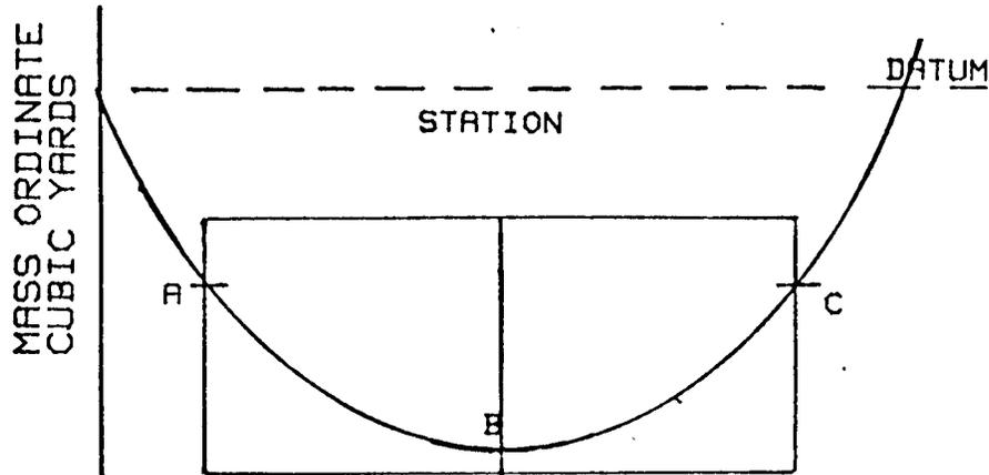
The vertical distance on the mass diagram between station A and station B is the yardage of fill generated between the two stations.
