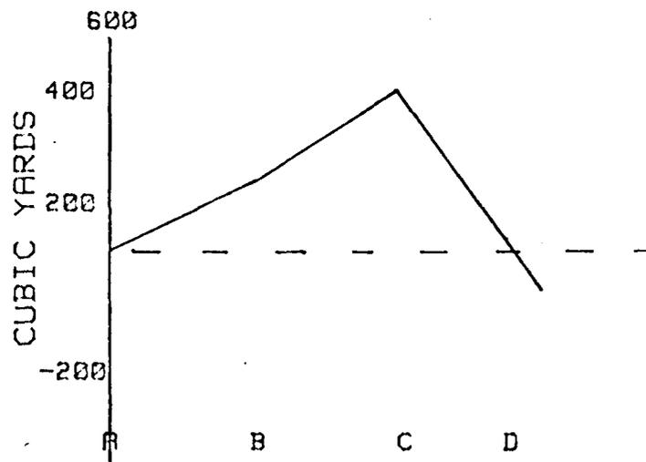
A couple of rules of thumb will assist the designer in preparing the mass diagram for a project. In the preliminary stages of the design the horizontal scale for the mass diagram should be the same as the horizontal scale for the profile. During the analysis of the mass diagram it will be easy to compare the mass diagram to the
